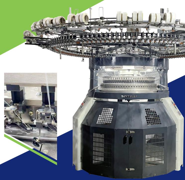
With 2 track dial cams & 4 tracks cylinder cams setting
